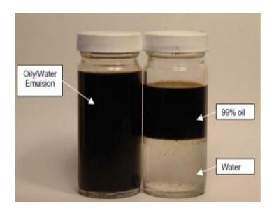
SF-F used to separate Oil and Water Emulstions
