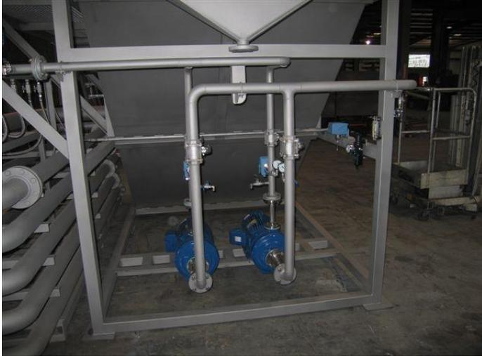
In the Pipe Flocculator, the microscopic air bubbles attached themselves to the chemically flocculated waste particles, making them strongly buoyant. The Pipe Flocculator inlet distribution header provides a uniform flow of the flocculated wastewater into the DAF Whitewater System flotation cell.
