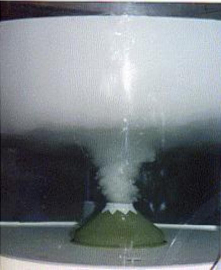
The injection of air results in Whitewater which is pumped through the innovative Pipe Flocculator. The Whitewater contains millions of microscopic tiny air bubbles. Extensive laboratory evaluation on the size of the air bubble and effective liquid-solid separation, overwhelming demonstrate that the smaller the air bubble, the more efficient the separation.
