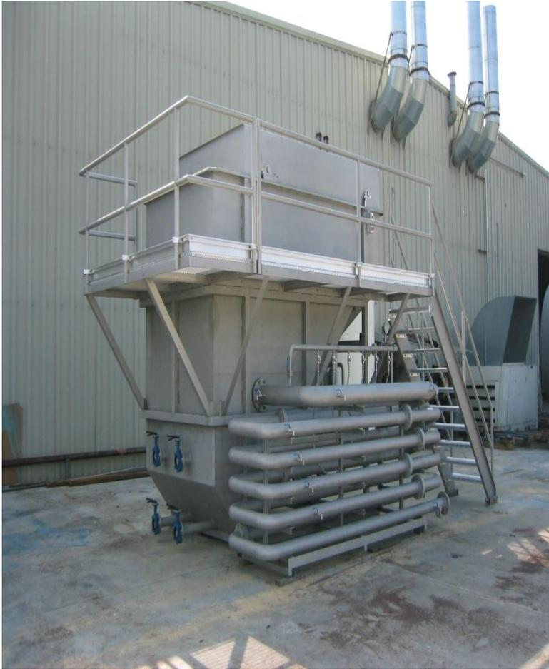
The **DAF Whitewater System** technology was developed by Water Resources utilizing the Patented Shearforce technology. The heart of the system is the ability of the Shearforce Pumps to pump gas/air which has been injected into the suction of the pumps. The unique Shearforce design allows the pump to pump gas/air without concern for solids or cavitation found in other pumps capable of pumping gas.
